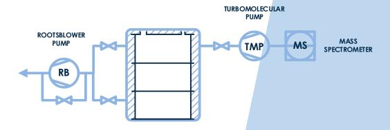
While the vacuum leak tester is already a proven solution for fast and accurate testing of steel drums, the **Helium Detection Add-On** improves its performance and precision, without replacing the core system.
